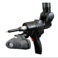
Elaser scanner accuracy according to manufacturer's test procedure determined by scanning a plane from various directions, each time using the entire sensor field of view depth, width and diagonal. The result is the maximum 1 $\sigma$  deviation of the scan data to fitted plane features.
